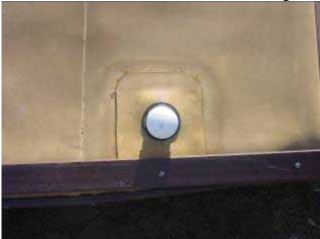
Figure 8. Modification to STAPP, access port to water collection reservoir tube.
