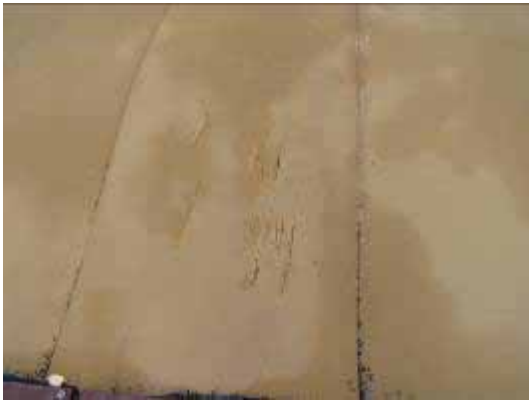
Figure 7. 7.62mm rounds pass in and out of the STAPP membrane
