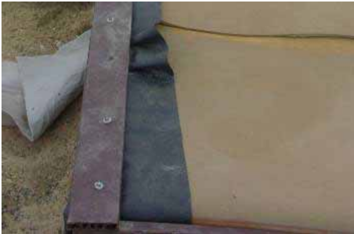
Figure 3. Liner and upper membrane attached to frame.
